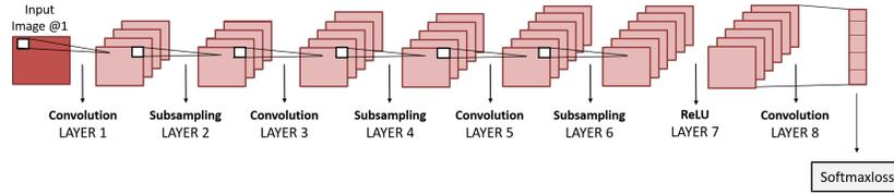
**Fig. 7.** Architecture of the convolutional neural network for emotion recognition in images**Table 2.** Architecture parameters in the convolutional neural network for each experimental scenario
